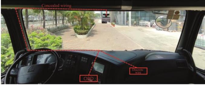
The **VT3500** is equipped with a power supply box which has a built-in switch control. Therefore, the power supply box needs to be fixed to a certain position within the vehicle. Please pay attention to the following tips when choosing the fixed position:
