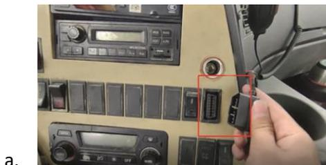
2. If connecting to the power supply via the vehicle's internal wiring, connect POWER/ACC/GND with the respective vehicle power cable.
