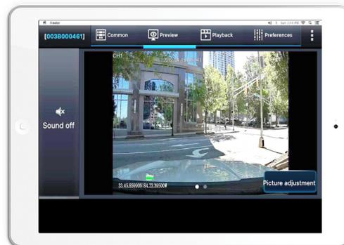
Adjust external facing camera with wrench and screw on device to see exterior surroundings. Play the video of channel 1 on MiFleet + Vision device through the Veyes Application. Adjust lens up and down until screen is at optimal viewing. Complete same steps for internal facing camera.
