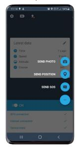
Report messages are saved to the "Black box" until they are ready to be sent based on automated parameters. To manually send, click the **UP** arrow button at the top of the screen, and then select **UNLOAD** when prompt.
